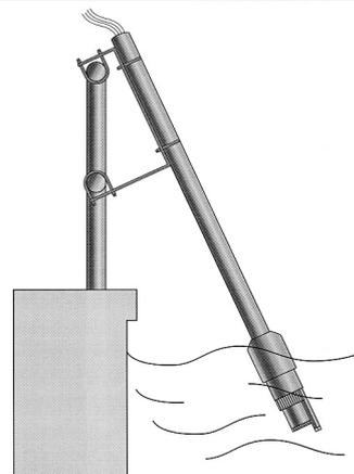
Typical installation of the submersible sensor.
