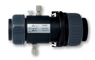
For very precise measures and low Turbidity values, as required by most drinking water application, we suggest to install the probe in the overflow cell **TU 910**.
